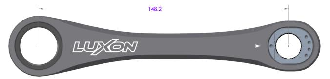
3) Inserts are identified by different numbers of dots on each end, and the pull-rod length is determined by the laser etched arrow pointing to the dots. Refer to the chart below for the resulting length at different adjustment positions. The image above shows the insert installed with the arrow pointing to one dot, which results in a 148.2 mm long pull-rod.
